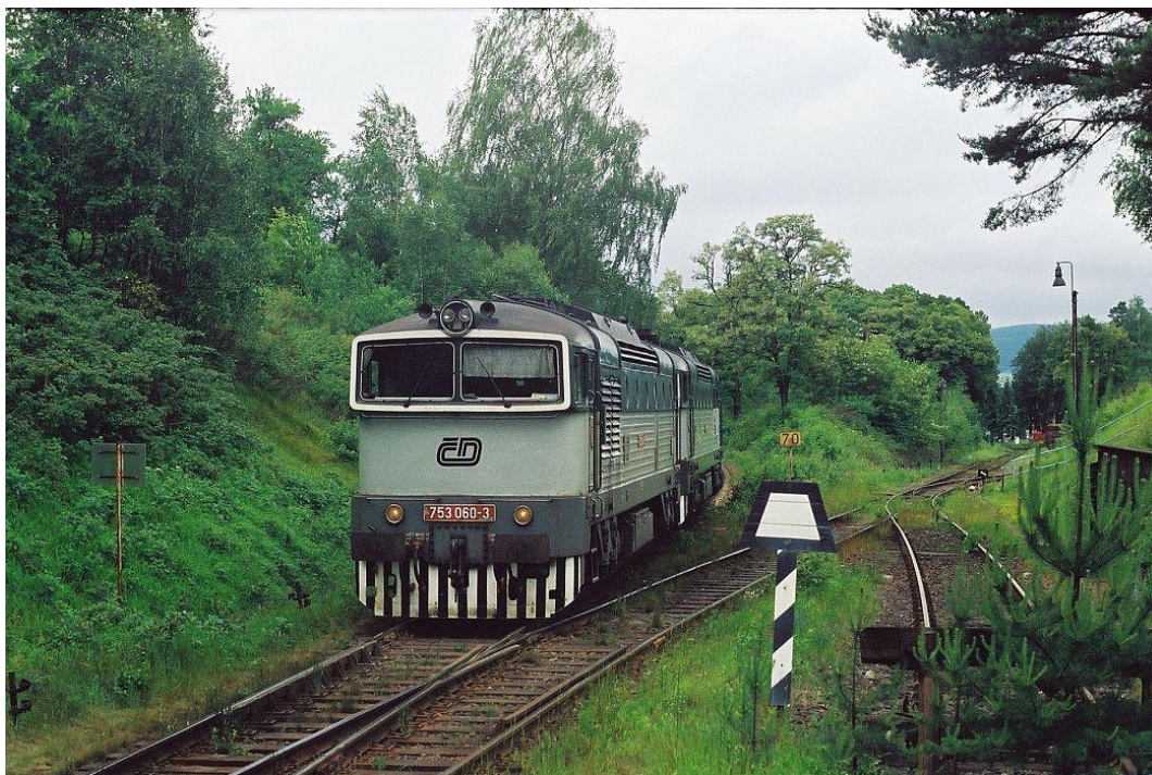
Picture: The trapezoid sign board in the front is the border of operating post D3 Havlovice located near to branch Pasečnice, where the regional line to Planá u Mariánských Lázní depart from the main line from Pilsen – Domažlice to Česká Kubice – Furth im Wald (Bavaria) (photo: Tomáš Paška, www.strojvedouciplzen.cz )
