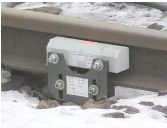
Picture: Axle counters (photo: SŽDC)
