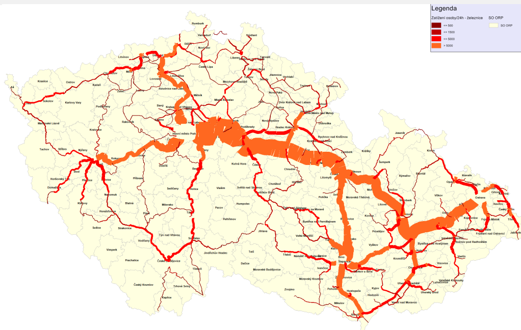
Figure 6.5 – Volume flow diagram of the load with railway passenger transport, transport model 2010
