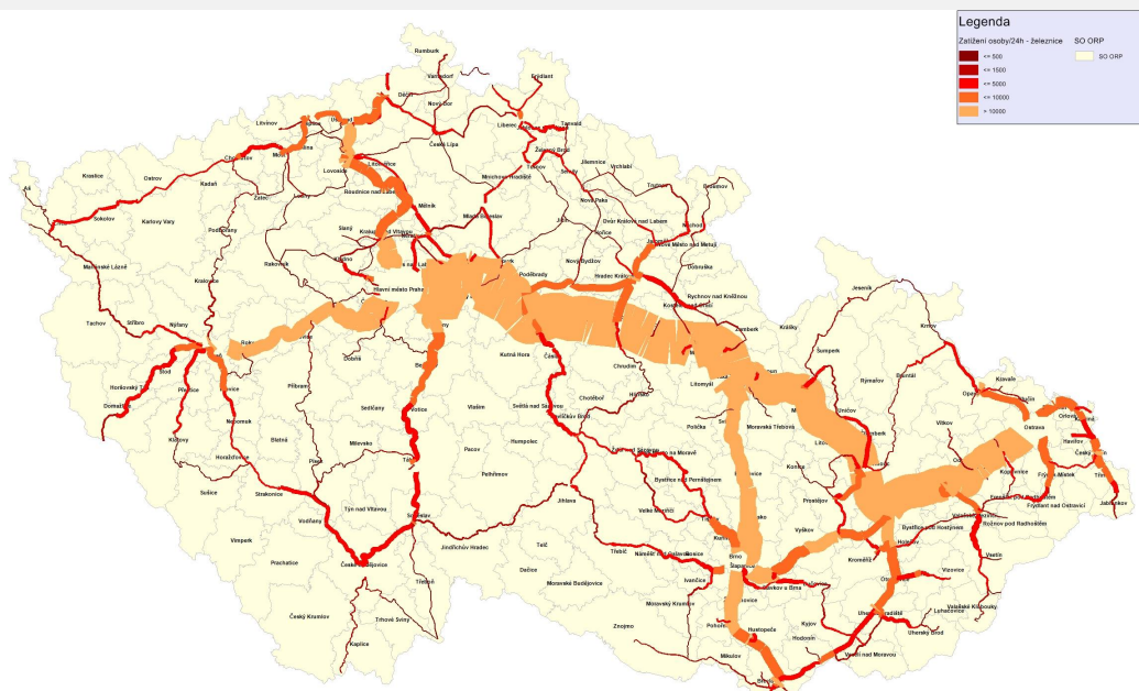
Figure 14.9 – Volume flow diagram of the load with railway passenger transport, transport model 2050, persons/24h
