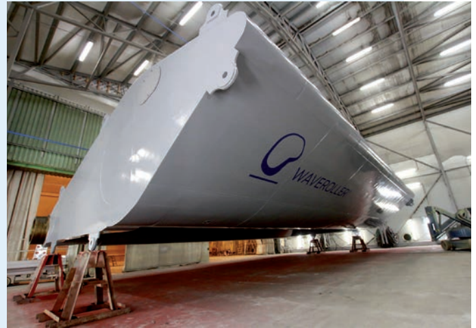
Figure 10: Production of a WaveRoller blade for a 350kW demonstrator. © AW-Energy
